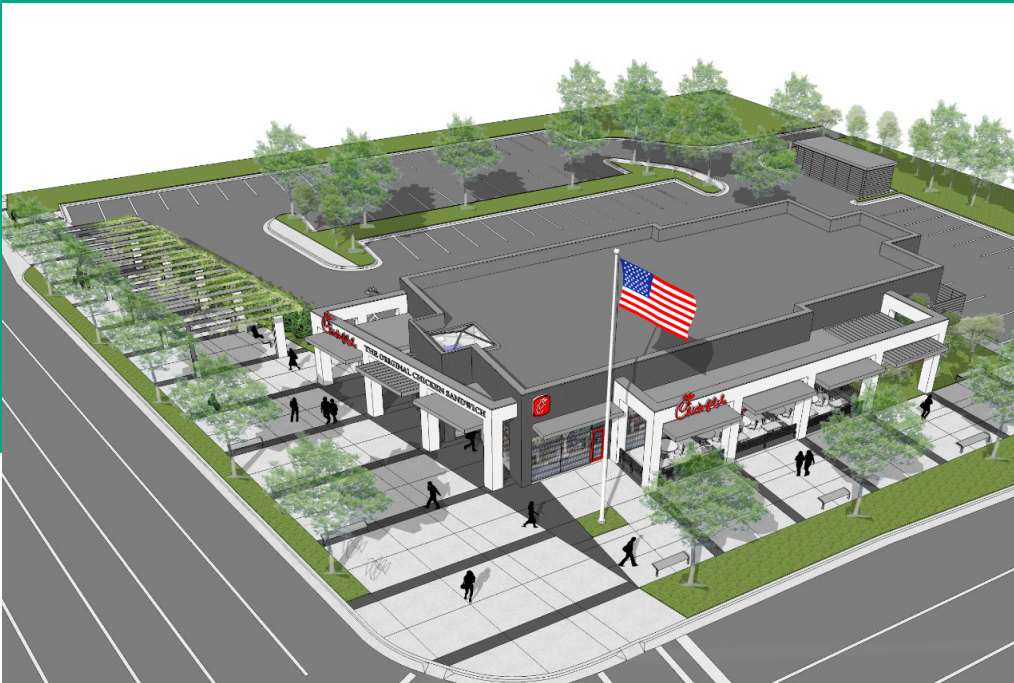
A bird's-eye perspective shows the 5,700-square-foot structure wrapped with arcades fronting 20th Street and Highland Avenue. New sidewalks extend to the building fronts. A trellis and landscape edge (left) extend a pedestrian envelope past the side/rear parking.
