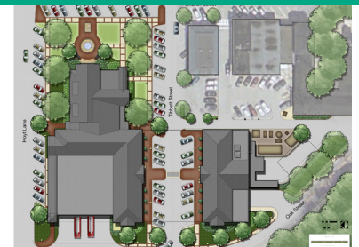
As the site plan shows, the design team managed to fit four times the space on the site of the former municipal buildings. Below-grade employee parking extends under Tibbett Street between the fire and police departments.
