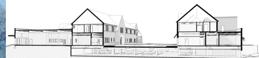
A single level of parking extends across the middle rear of the site between the fire department/city hall (left) and police department.
